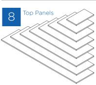
Top Panels overhang cabinets by 1/8", 3mm at the front and by 1", 25mm at the back to clear skirting boards. They add 7/8". 22mm to the height of the cabinets.
